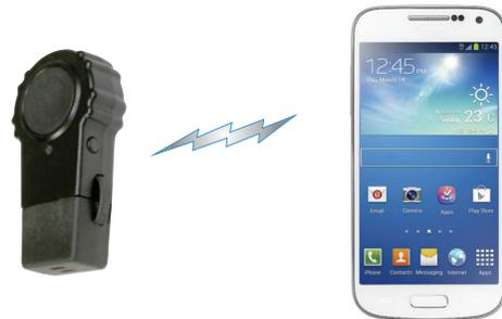
The BT-PTT2-ZD Push-to-Talk is designed to work with smartphones running the Android operating system. Prior to normal operation, the phone and Push-to-Talk must be *paired* together using the following process:
