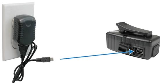
The PRYMEBLU Lapel Microphone has an internal Lithium Ion rechargeable battery pack which must be charged prior to operation, and must be recharged regularly. A fully charged battery will provide approximately 12 hours (or more) of operation before needing to be recharged. However, operating time can vary depending on usage and the condition of the battery pack. Recharge the battery regularly.
