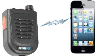
When pairing the PRYMEBLU Speaker Microphone with a cellphone, make sure that the speaker microphone and all other nearby Bluetooth devices are powered off before beginning.
