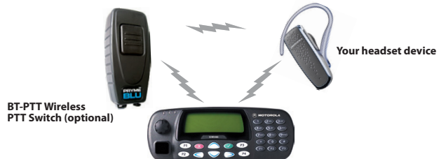
FIG. 4 - Wireless Communication System
