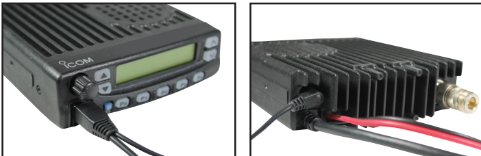
FIG. 3 Typical Front and Rear Connection Radio
