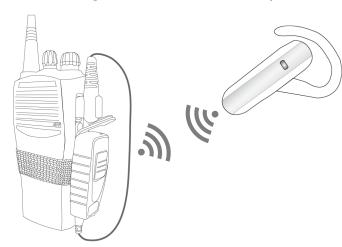
STEP THREE: Pairing with an Audio Accessory \*When pairing the PRYMEBLU Adapter with a headset, make sure that both the PRYMEBLU Adapter and the 2-way radio the adapter is connected to are both powered off Turn the power switch on the back of the PRYMEBLU Adapter to the ON position while holding down the Talk button on the front of the
