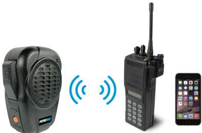
Connects wirelessly to PRYMEBLU® radio adapters, such as the BT-523
