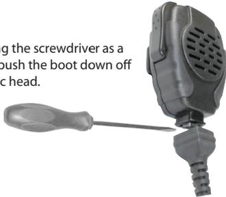
3. Once the boot is clear of the mic head, push it down the cable away from the microphone to expose the RJ45 (telephone handset style) connector.
