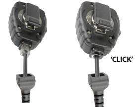
2. Push the RJ45 connector into the jack until the tab "clicks" and locks into place.
