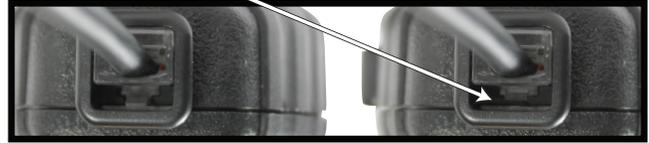
5. Once the tab had been pushed up, the cable should be "unlocked" from the microphone. Pull the cable out of the microphone head. The cable and microphone head should now be separate from each other.
