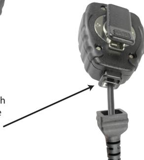
4. Insert the small flathead screwdriver under the locking tab of the RJ45 connector and push the tab up.
