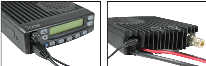
FIG. 3 Typical Front and Rear Connection Radio
