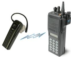
**STEP ONE:** When pairing the PRYMEBLU BTH-200 Bluetooth Headset with a PRYMEBLU Radio Adapter, make sure that the headset, two-way radio, and PRYMEBLU adapter are all powered off to start. To turn the headset off hold the Multifunction Button + the Volume Down button for three to four seconds.
