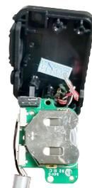
4. Remove the old battery from the battery holder. A ball point pen can be used to push the battery out of the holder if needed.
