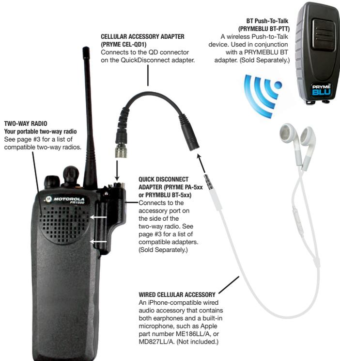
**NOTE:** Always power your two-way radio off when connecting or disconnecting any adapters or wired audio accessories.
