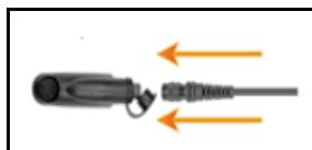
Quick Disconnect (QD) accessories and radio adapters provide both security and usability. Just install the PA series adapter onto the radio then plug the QD accessory into the rugged six-pin QD connector. **DON'T SEE WHAT YOU WANT? WE ARE ALWAYS ADDING NEW PRODUCTS - PLEASE CALL FOR THE LATEST INFO.**
